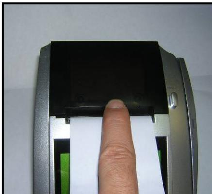
5. Carefully close the printer compartment so that it snaps firmly into place.
