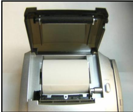
4. Insert the paper roll and spindle into the slot provided so that the paper is fed from the bottom of the roll and over the tear bar.
