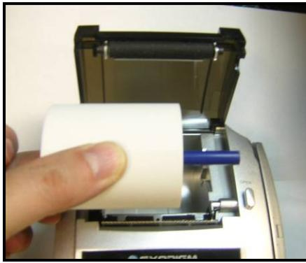
3. Place a new roll of thermal paper on the blue support spindle. Paper should have the shiny side to the outside of the roll.
