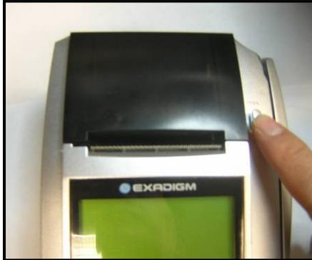
1. Open the paper compartment by pressing the OPEN button to the right of the paper cover. Grasp the cover on both leading edges and lift upward.
