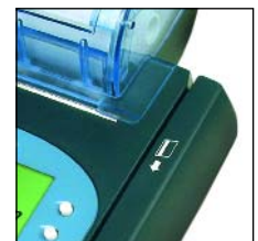
Standard Track 1, 2 & 3 magnetic stripe reader
