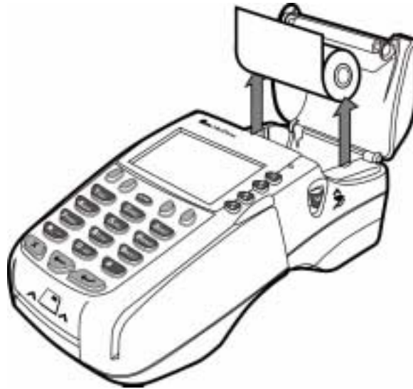
Figure 6 Removing Partial Paper Roll
