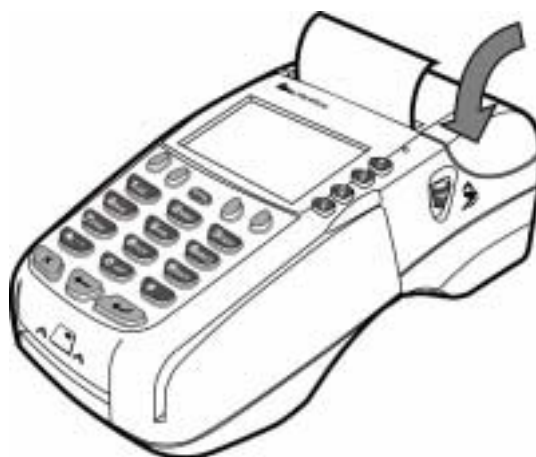
Figure 8 Closing Paper Roll Cover
