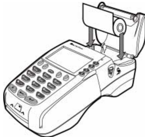
Figure 7 Loading Paper Roll
