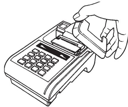
Figure 3-3. Removing the Printer Cover
